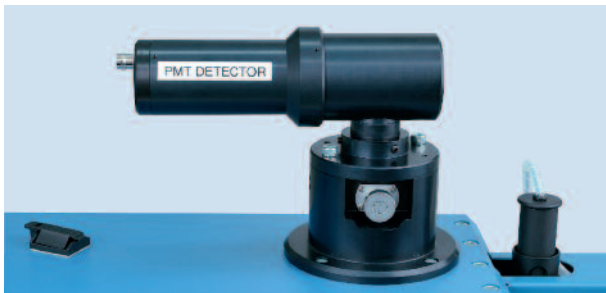
Vacuum-UV photomultiplier-tube (PMT) detector mounted on SpectroMaster® HR
