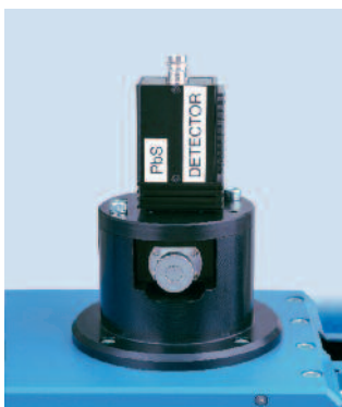
Thermoelectrically cooled PbS Infrared detector mounted on SpectroMaster® HR
