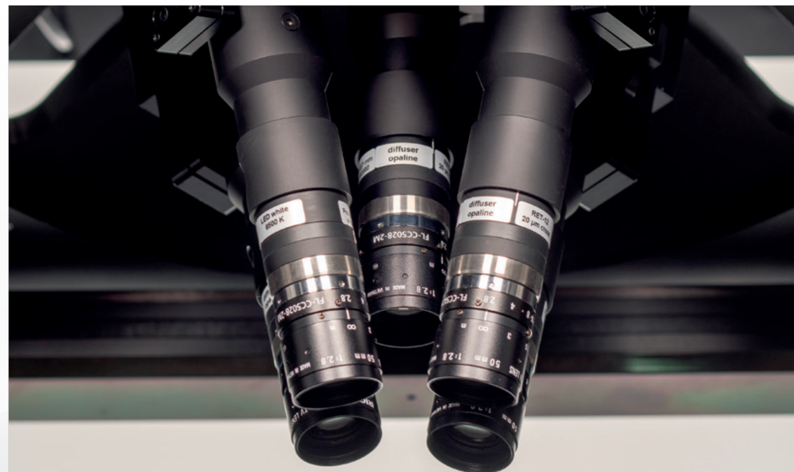
Configuration for narrow FOV camera testing
