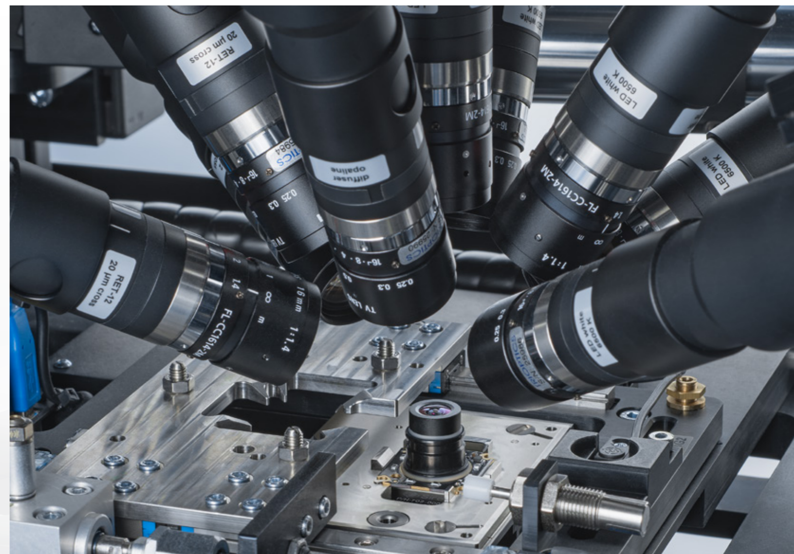
Configuration for narrow FOV camera testing
