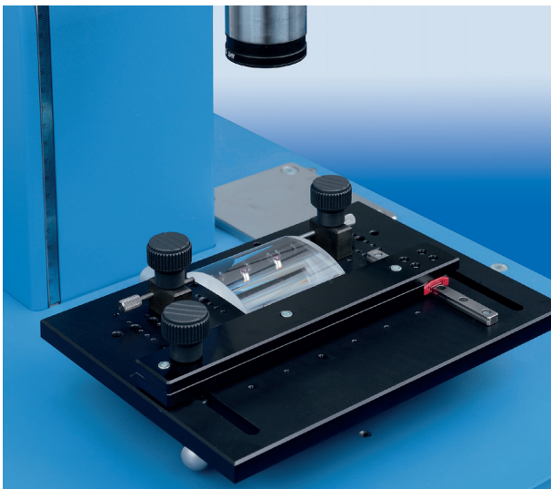
OptiCentric® 100 while measuring a cylinder lens
