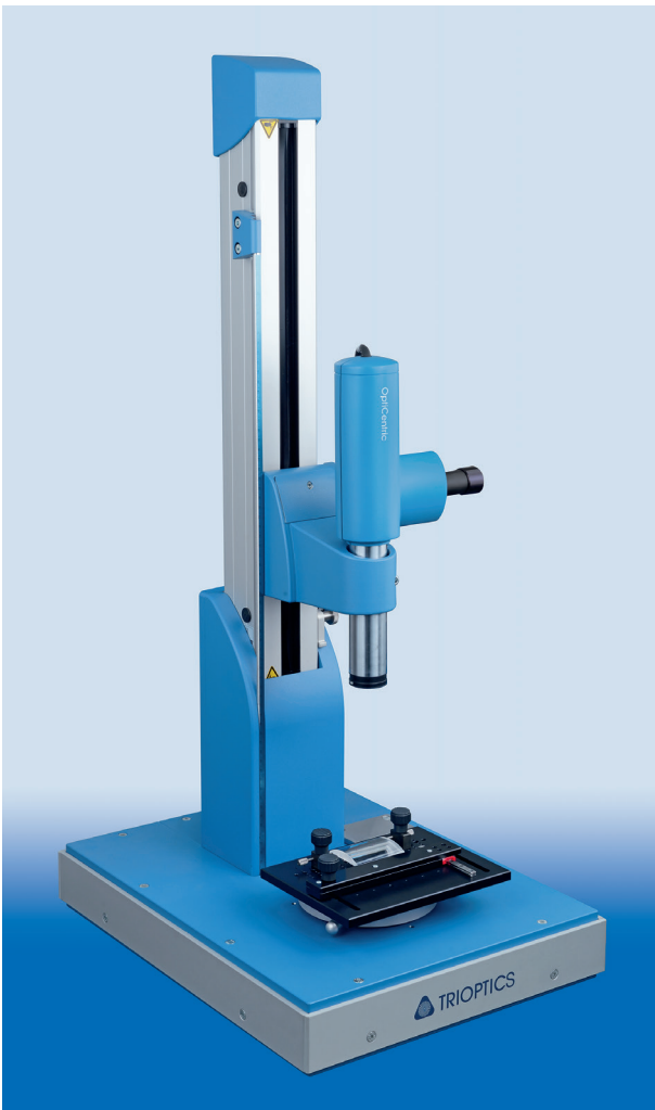
OptiCentric® 100 measuring a cylinder lens
