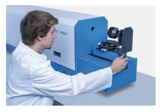
Centration testing with the OptiCentric® Linear technology is especially suited for position-sensitive objective lenses with e.g. integrated floating elements and can be performed in a horizontal setup.
